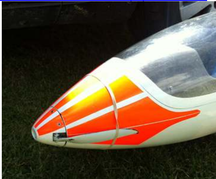
Woo’s FES installation in the front of a big FS1. Very neat.
